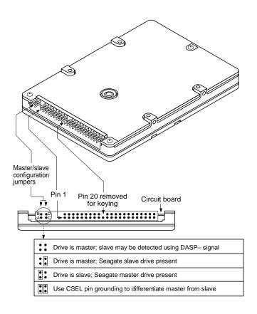
Figure 1. ATA interface connector and master/slave configuration jumpers
