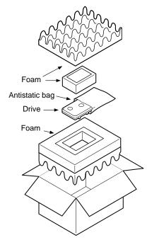
Figure 2. Seagate 2.5-inch drive and approved packing materials
